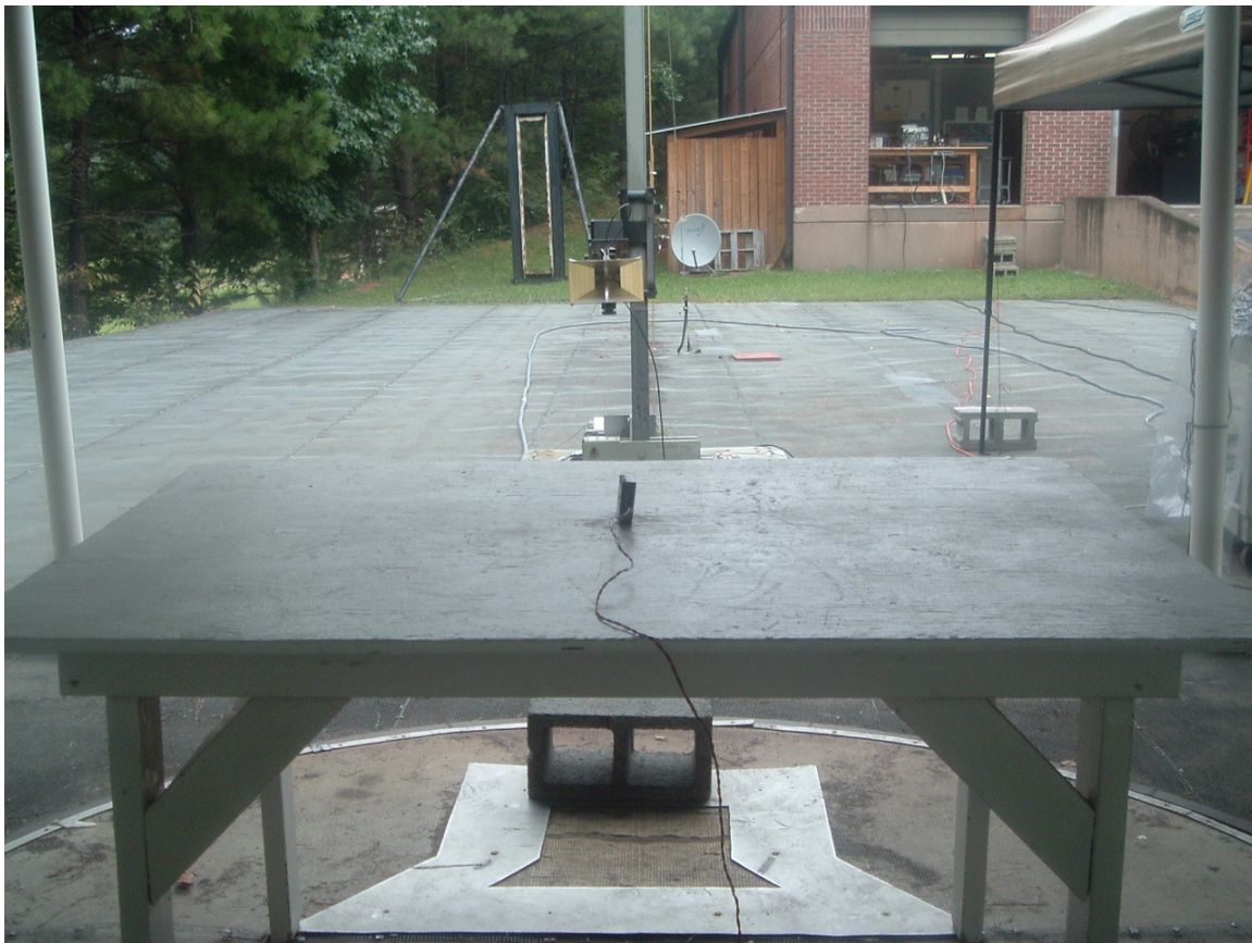
Figure 7. Radiated Emissions Test Setup Spurious Emissions testing in worse case position "Y".
