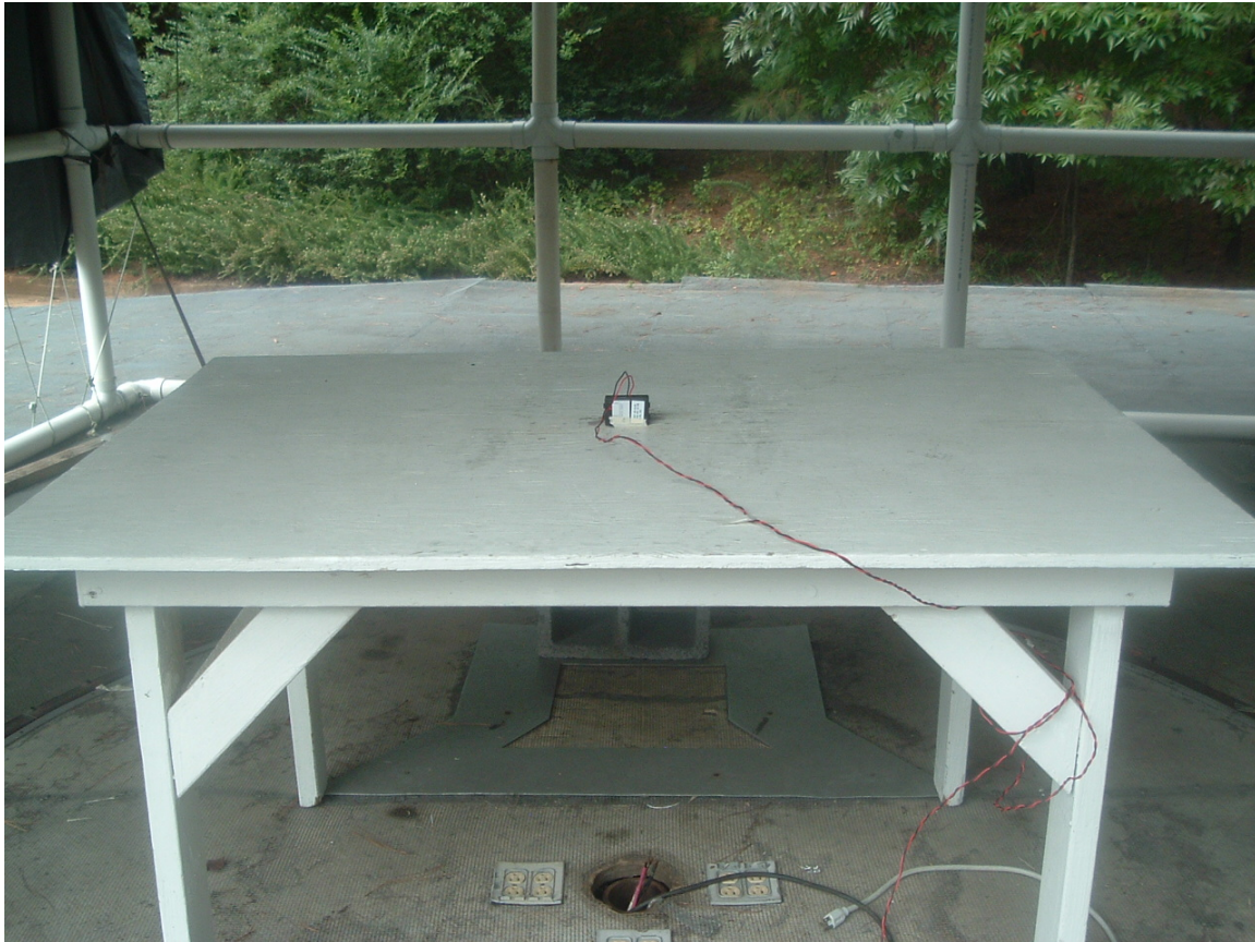
Figure 5. Radiated Emissions Test Setup Font view testing in Position "Z"
