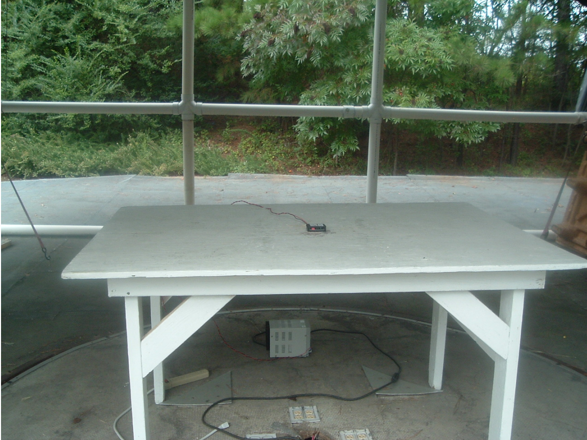
Figure 1. Radiated Emissions Test Setup Front view testing in position "X"
