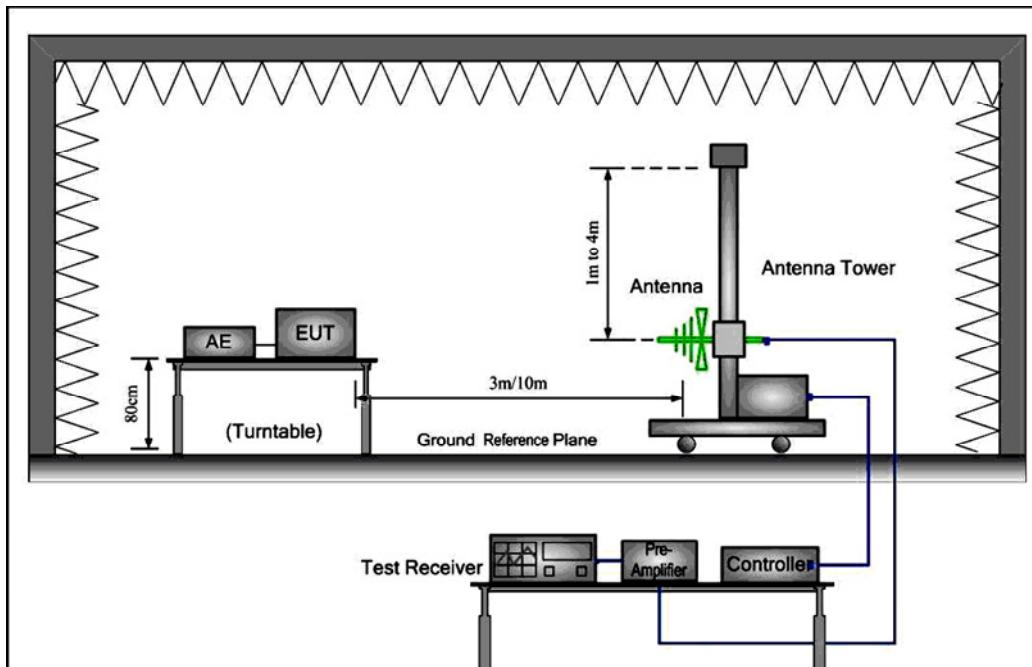
**1) Fundamental emission:****Antenna polarization: Vertical:**
