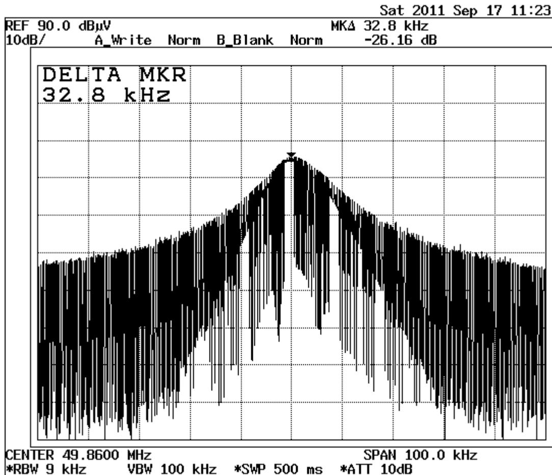
Result : The field strength of any emission within the operation band did not exceed 80 dB( $\mu$ V/m) for average value or 100 dB( $\mu$ V/m) for peak value. Refer to page 9 for the recorded value for the emission at the fundamental frequency.
