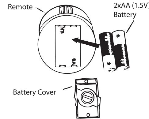
Insert two AA batteries (not included) and replace door.
