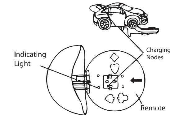
To charge the car, open the cover at the bottom of the controller. Align metal nodes on controller with the nodes on the car and place car onto the controller. The charging indicator light will come on when the car is charging. After a full charge (approximately 2-3 minutes) the light will turn off.
