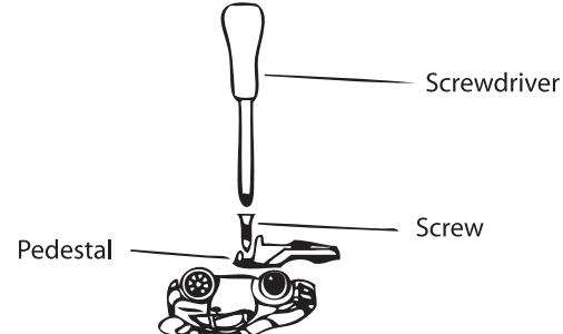
Use a screwdriver to detach the car from the battery cover and pedestal.
