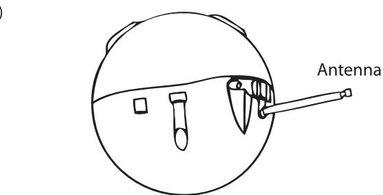
Place antenna into hole at the top of controller.
