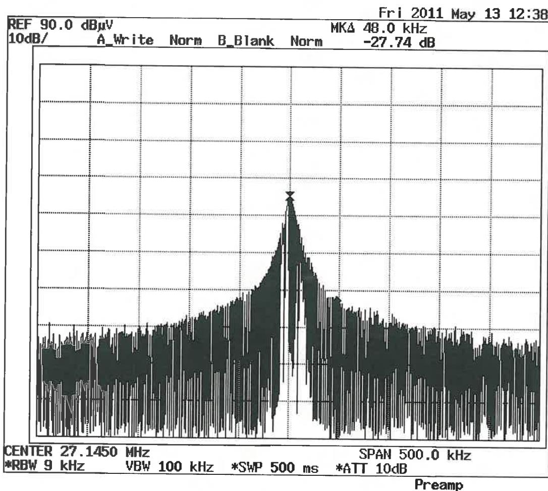
Result : The field strength of any emission within the operation band did not exceed 80 dB( $\mu$ V/m) for average value or 100 dB( $\mu$ V/m) for peak value. Refer to page 10 for the recorded value for the emission at the fundamental frequency.
