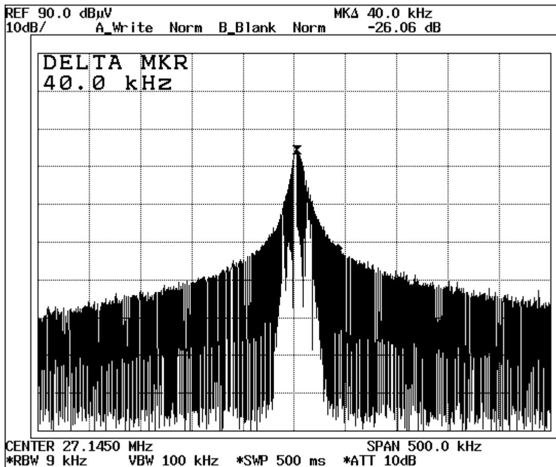
Result : The field strength of any emission within the operation band did not exceed 80 dB( $\mu$ V/m) for average value or 100 dB( $\mu$ V/m) for peak value. Refer to page 10 for the recorded value for the emission at the fundamental frequency.
