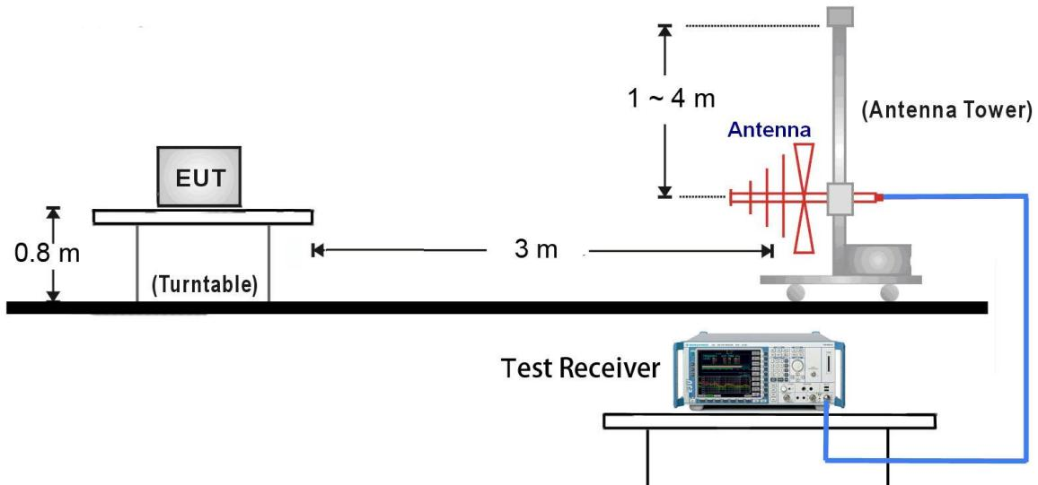
1GHz ~ 18GHz Test Setup:
