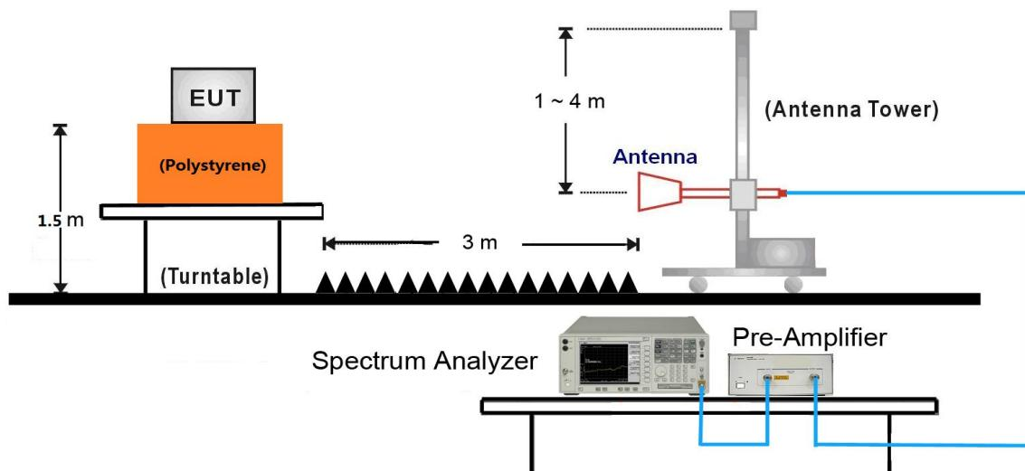
18GHz ~25GHz Test Setup:
