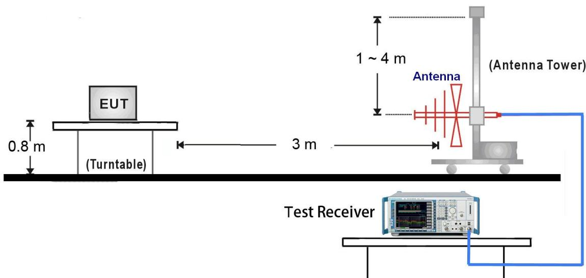
1GHz ~ 25GHz Test Setup:
