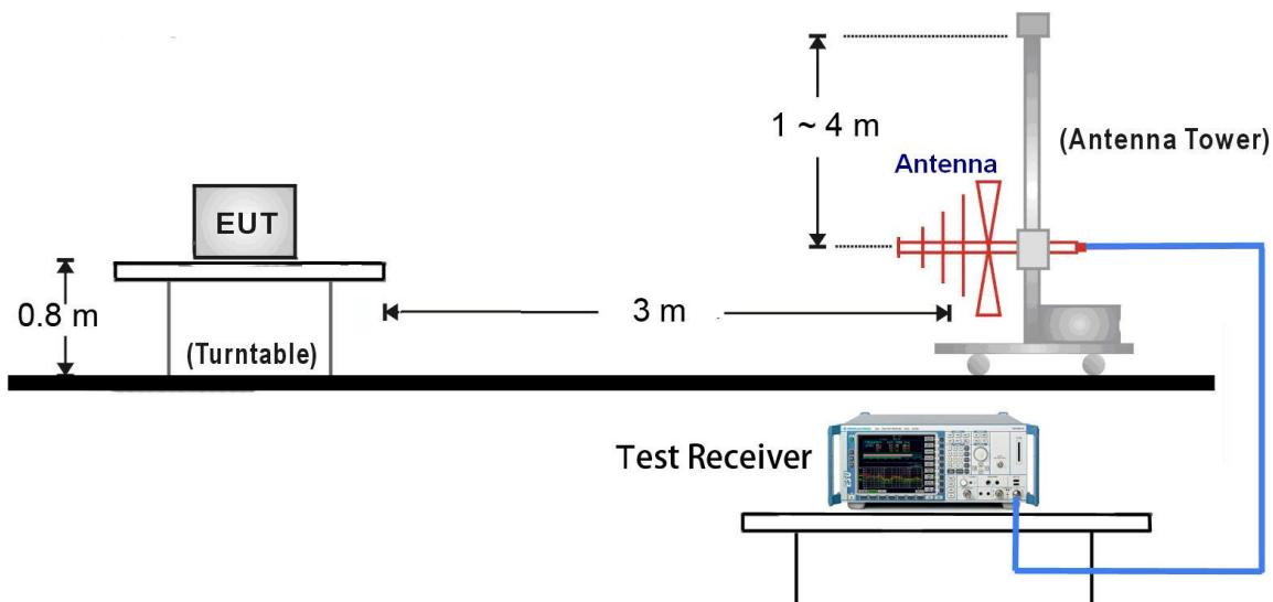
1GHz ~ 25GHz Test Setup:
