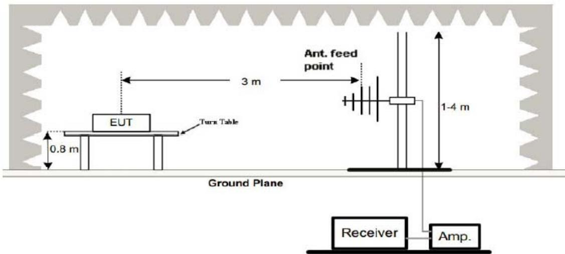
(3) Radiated Emission Test-Up Frequency Above 1GHz
