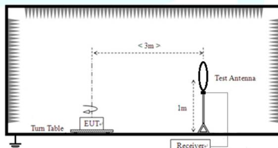
For radiated emissions from 30MHz to 1GHz
