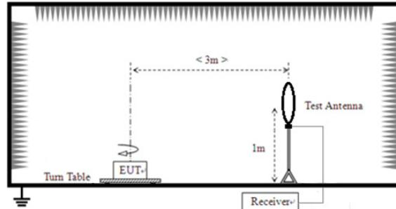
For radiated emissions from 30MHz to 1GHz
