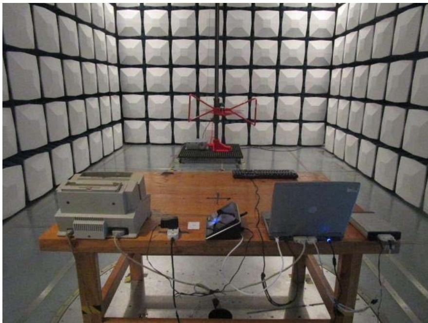
Radiated Emissions Below 1GHz –Rear View
