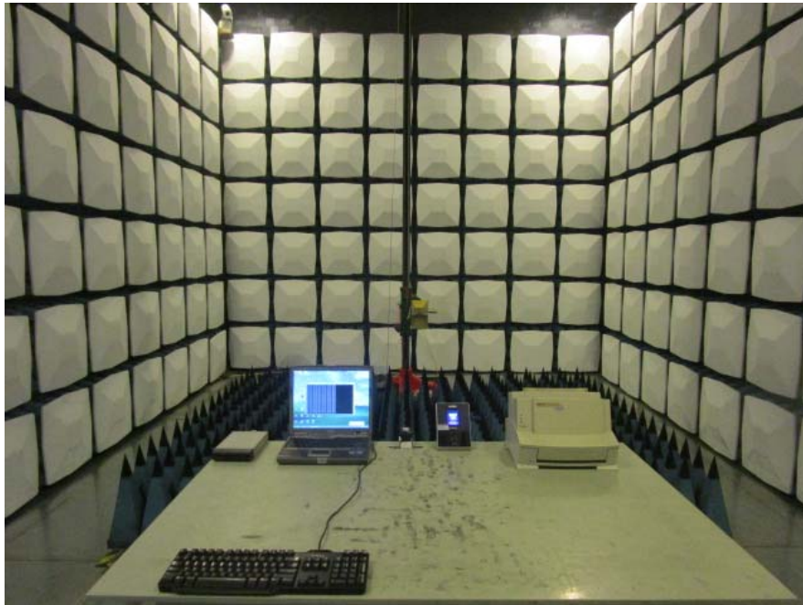
Radiated Emissions Above 1GHz - Front View
