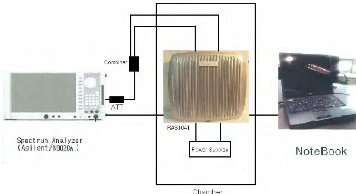
The center of the spectrum analyzer was set to block edge frequency.
