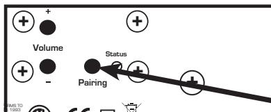
**D]** Set the Power switch, located on the back panel of your subwoofer, to “ON”. While the lights are still flashing on the transmitter, push the “pairing button” on the back panel of your e<sup>2</sup> Wireless SubWoofer. When the “STATUS” LED turns from Red to Green the pairing is complete.
