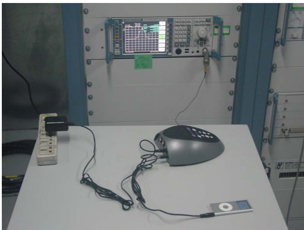
Set-up for 6dB and 99% bandwidth test
