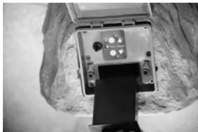
**Step 2:** Be sure the zone switch on the back of your AudioRock is set to zone 1 unless you are setting up a 2 Zone system. If you intend to set up a two zone system be certain the zone switch is set the number corresponding to the zone you intend to place it.
