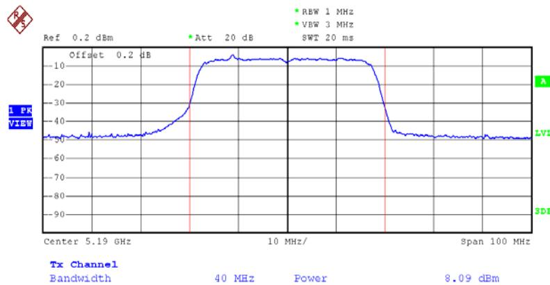
**Peak Conducted Output Power Plot on Configuration Draft n 40MHz ANT. A-1/5230**
