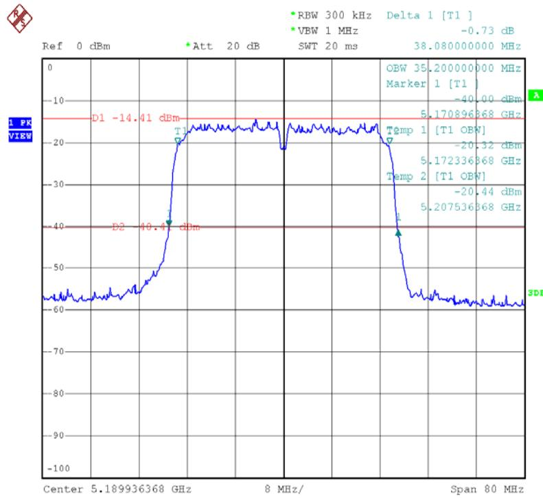
**26dB Bandwidth Plot on Configuration Draft n 40MHz ANT. A-1+A-2/5190MHz**
