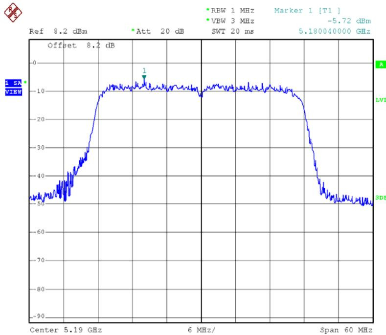
**Power Density Plot on Configuration Draft n 40MHz ANT. A-1+A2/5230**
