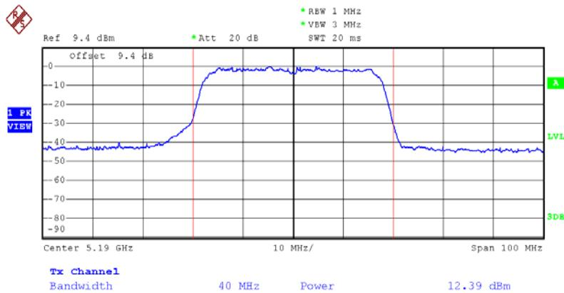
**Peak Conducted Output Power Plot on Configuration Draft n 40MHz ANT. A-1+A2/5230**
