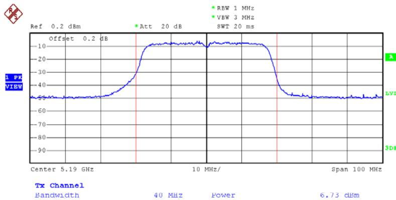
**Peak Conducted Output Power Plot on Configuration Draft n 40MHz ANT. A-2/5230**
