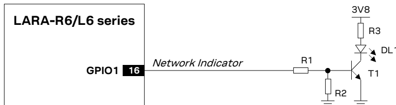
Figure 59: Application circuit for network indication provided over GPIO1
