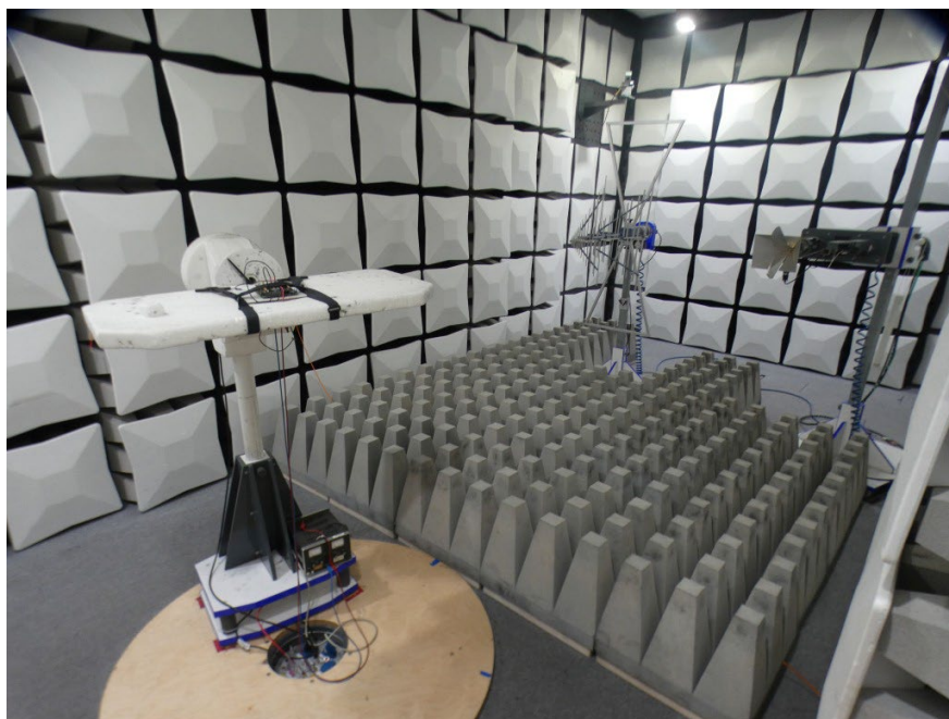
Photo 1: Test setup for radiated measurements above 1GHz
