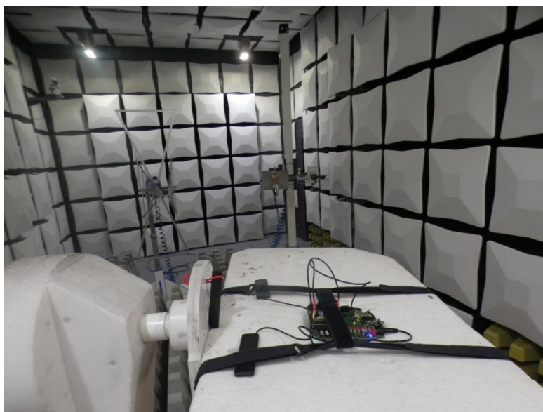
Photo 1: Test setup for radiated measurements
