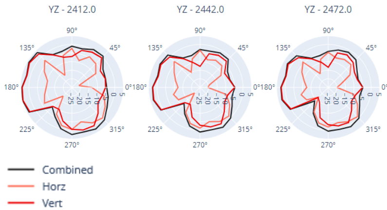
Figure 8: ANT-X100P001B24553 antenna – 2.4 GHz, 2D Y-Z plane radiation pattern
