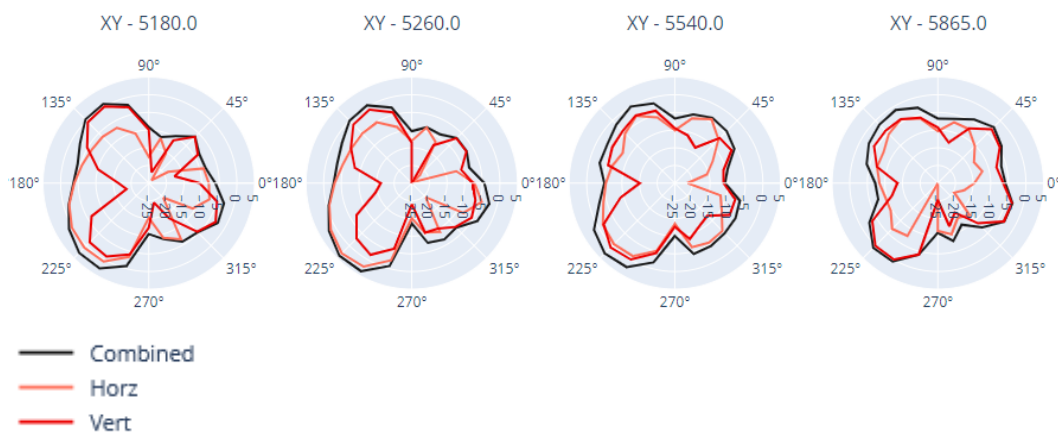
Figure 5: ANT X100P001B24553 antenna – 5 GHz, 2D X-Y plane radiation pattern
