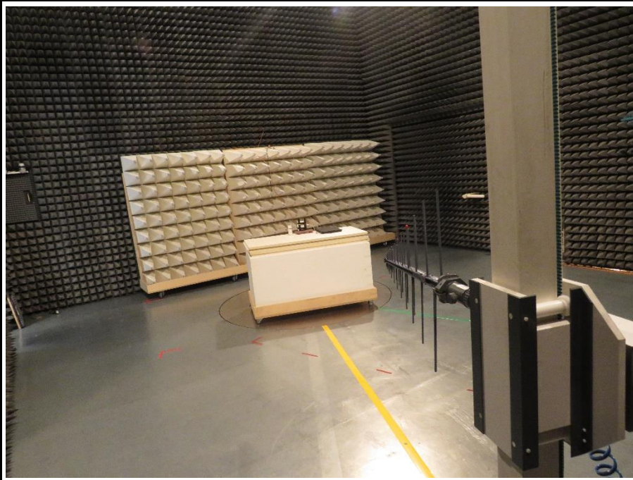
Setup below 1 GHz for Variant 2 (NORA-W101 with external antenna PN PRO-IS-237) -B
