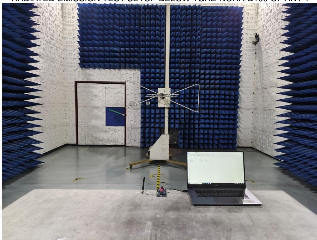
**RADIATED EMISSION TEST SETUP BELOW 1GHZ-NORA-B100 OF ANT 2**
