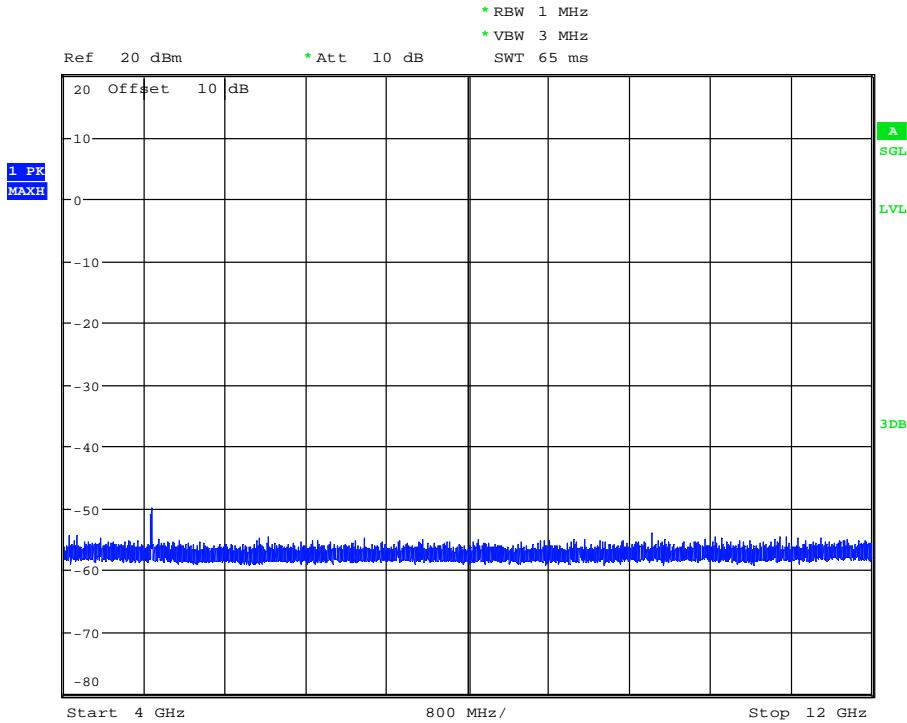
170297\_SpurEmiss12-18G\_b\_6.wmf: conducted spurious emissions (operation mode 2):
