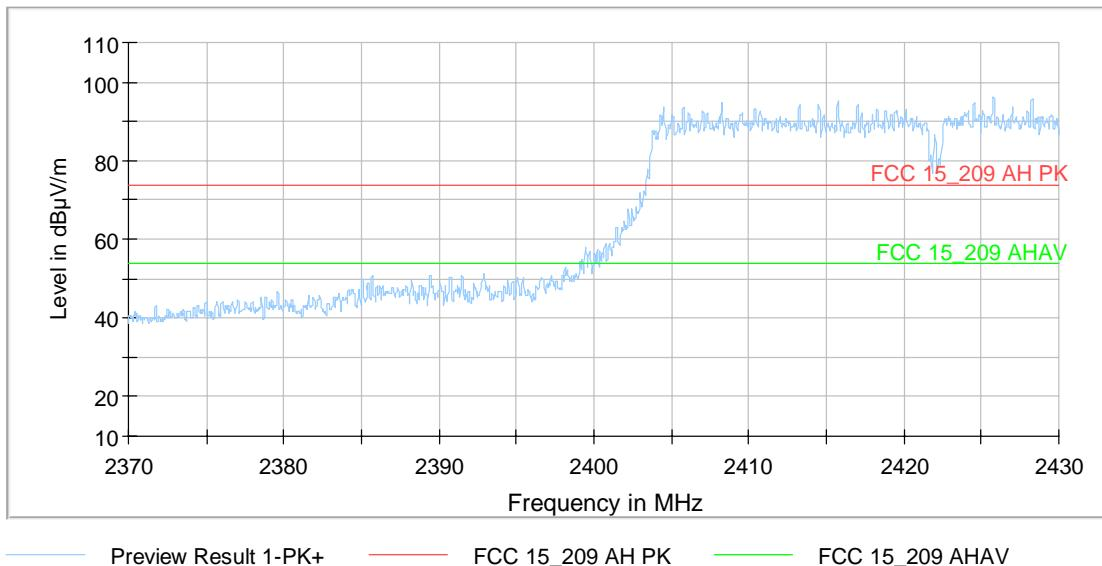
**Transmitter operates at the lower end of the assigned frequency band (operation mode 13)**
