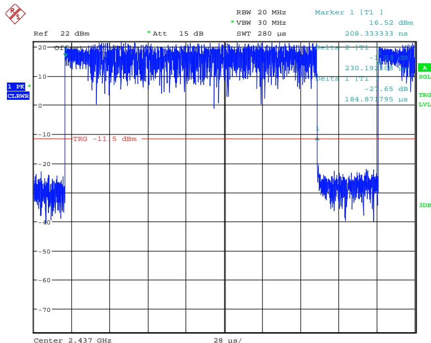
$$T_{TX\_on} = 184.9 \text{ ms}, T_{TX\_Period} = 230.2 \text{ ms} \quad (1)$$
