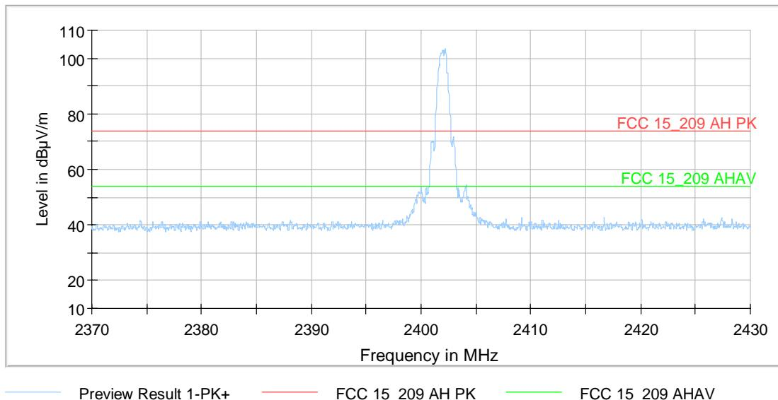
**Transmitter operates at the lower end of the assigned frequency band (operation mode 10)**
