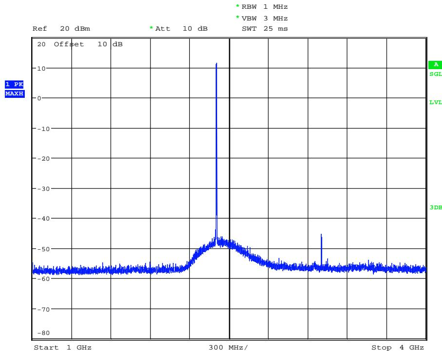
170297\_SpurEmiss4-12G\_BT\_DH5\_BT1.wmf: conducted spurious emissions (operation mode 1):
