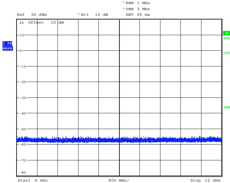
170297\_SpurEmiss12-18G\_BT\_DH5\_BT1.wmf: conducted spurious emissions (operation mode 1):
