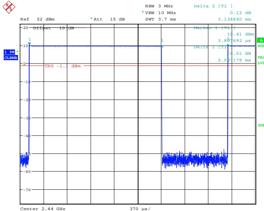
$$T_{TX\_On} = 2.087ms, T_{TX\_Period} = 3.125ms \quad (4)$$
