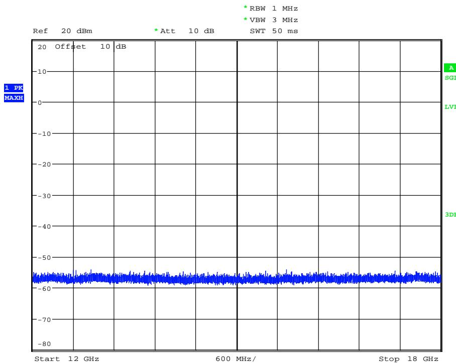
170297\_SpurEmiss18-26G\_BT\_DH5\_BT1.wmf: conducted spurious emissions (operation mode 1):
