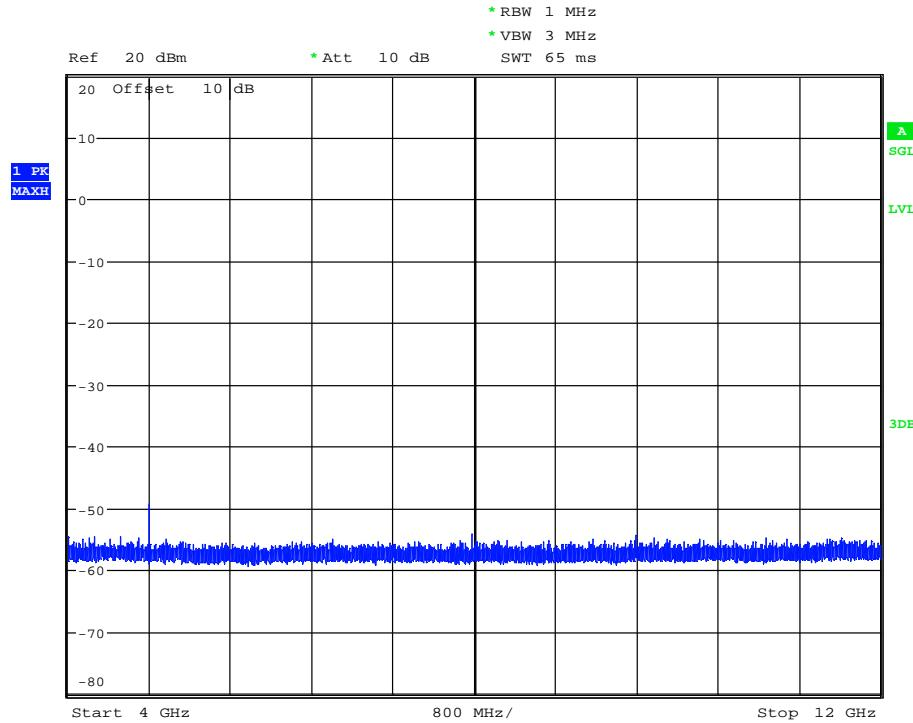
170297\_SpurEmiss12-18G\_BTLE\_BT1.wmf: conducted spurious emissions (operation mode 10):
