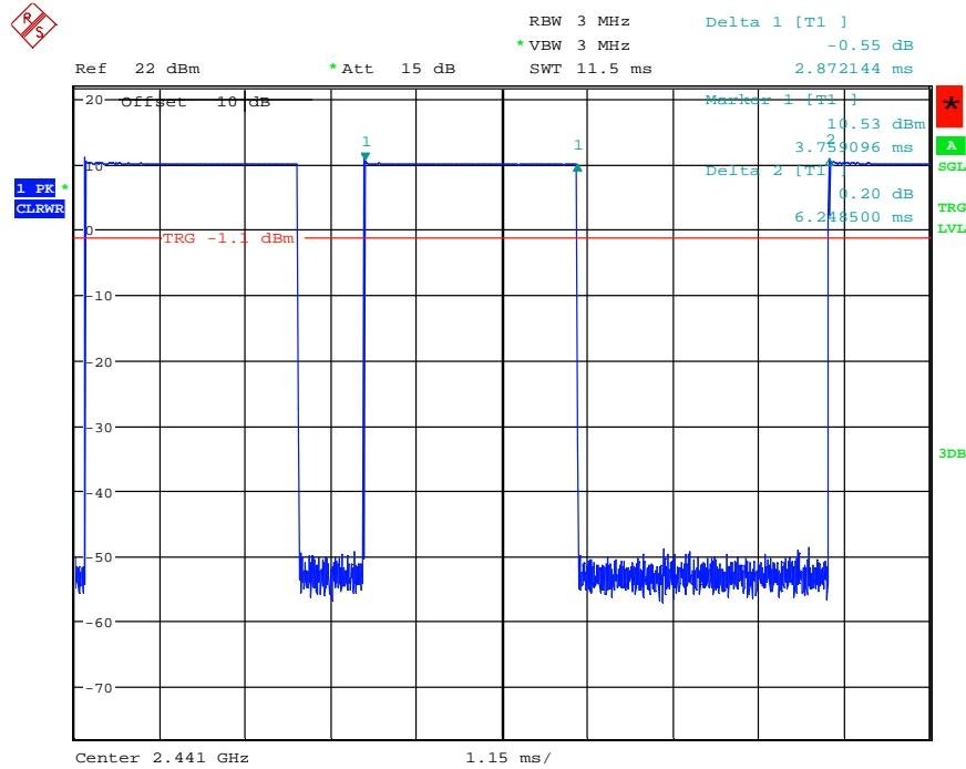
The signal combination was repeated after a short and a long Tx Cycle. Therefore the duty cycle could only be evaluated correctly, by looking at two consecutive TX periods.
