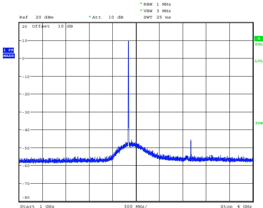
170297\_SpurEmiss4-12G\_BTLE\_BT1.wmf: conducted spurious emissions (operation mode 10):
