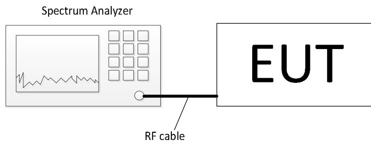
The relating measurements were carried out in a conducting manner. Therefore, the antenna connector was directly connected to a spectrum analyzer. The measurement procedure refers to part 11.11.2 and 11.11.3 of document [1].
