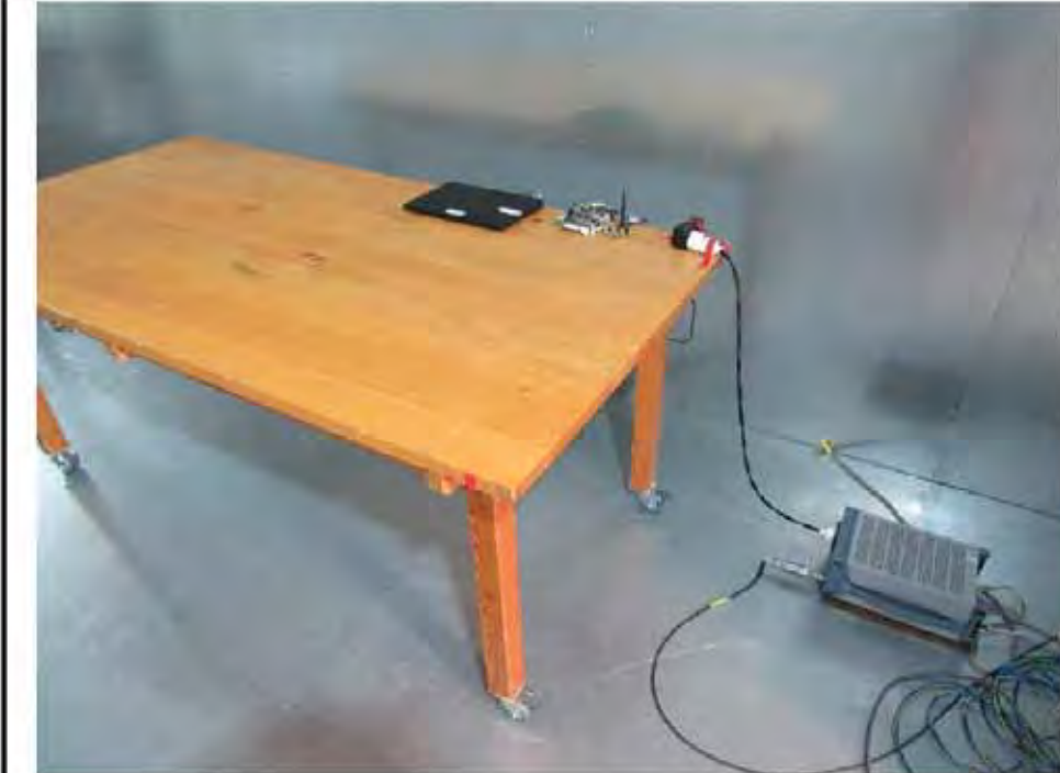
Setup for measurements 150 kHz - 30 MHz
