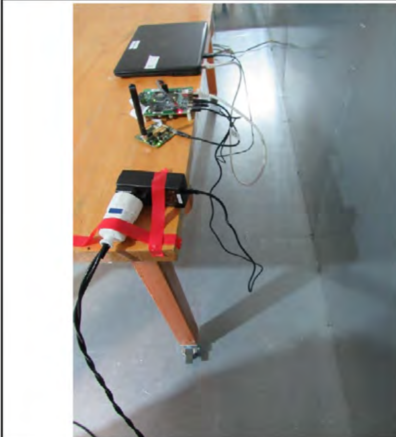
Setup for measurements 150 kHz - 30 MHz (cables)
