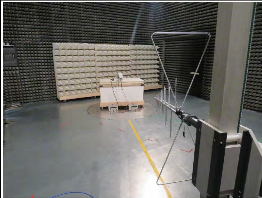
Setup for measurements below 1 GHz
