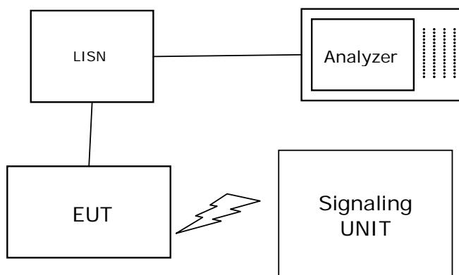
Setup in the shielded room for conducted measurements at AC mains port
