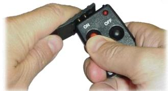
3. Press the metal pins on the RF Transmitter onto the two connection points on the MRD and hold them in this position.
