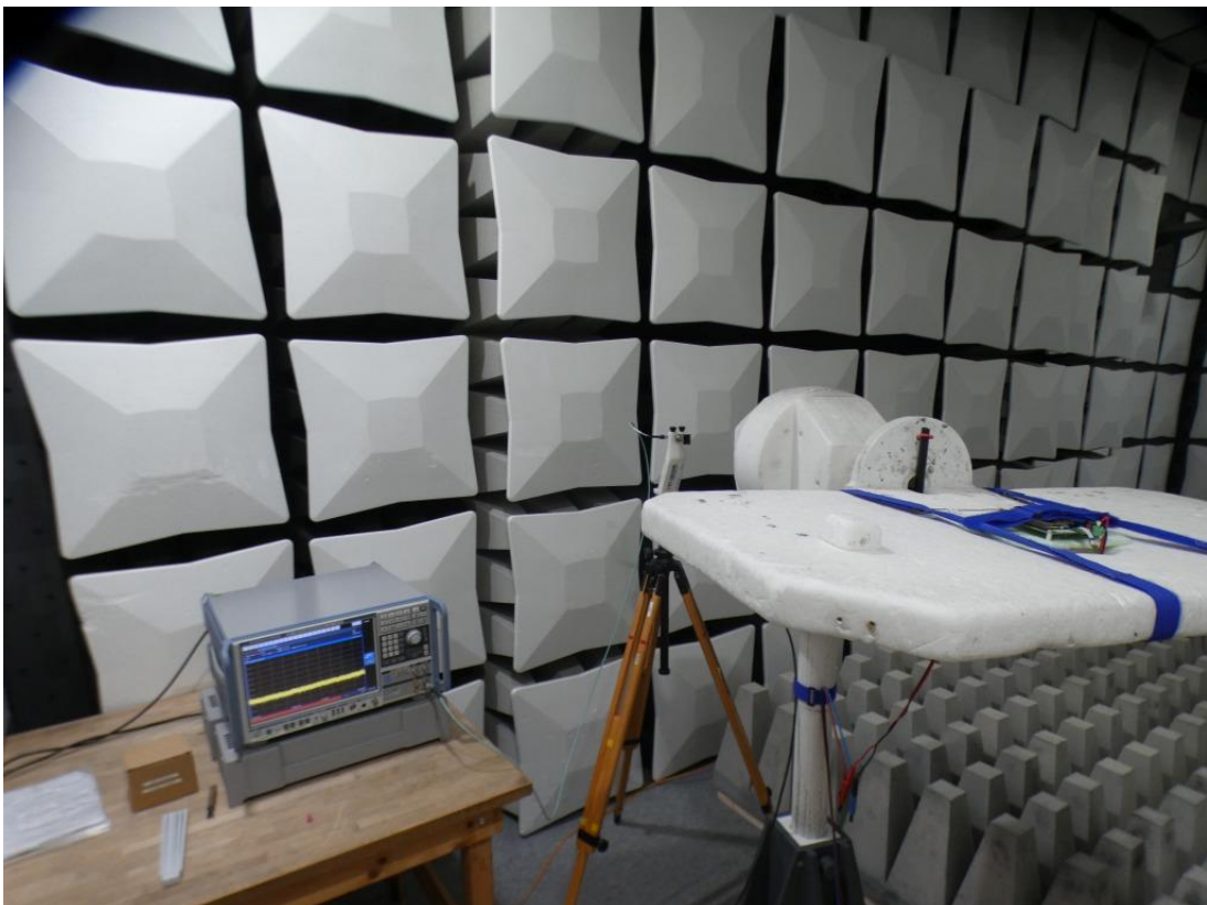
Photo 4: Test setup for radiated measurements above 26 GHz
