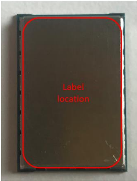
Figure 7: Label location of the JODY-W3 modules
