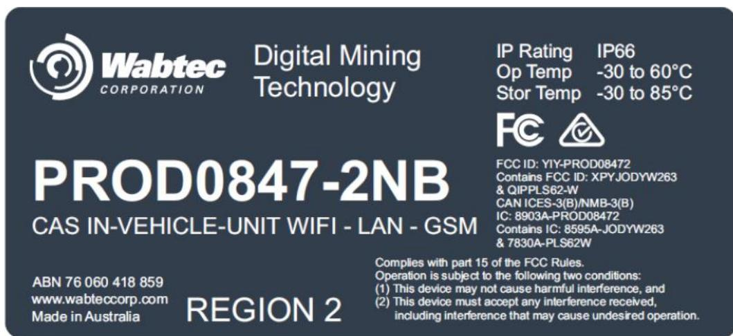
Label is affixed to the underside of the respective model, which is visible to the professional installer during vehicle installation.
