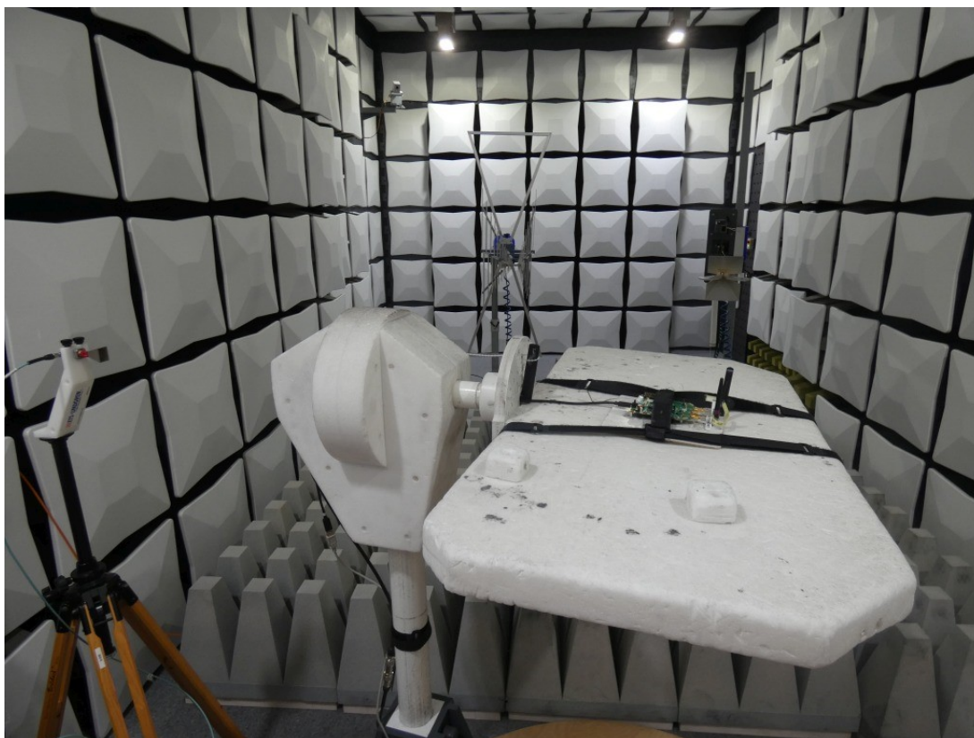
Photo 4: Test setup for radiated measurements above 26 GHz
