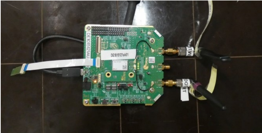
Photo 5: Test setup for radiated measurements EUT detail
