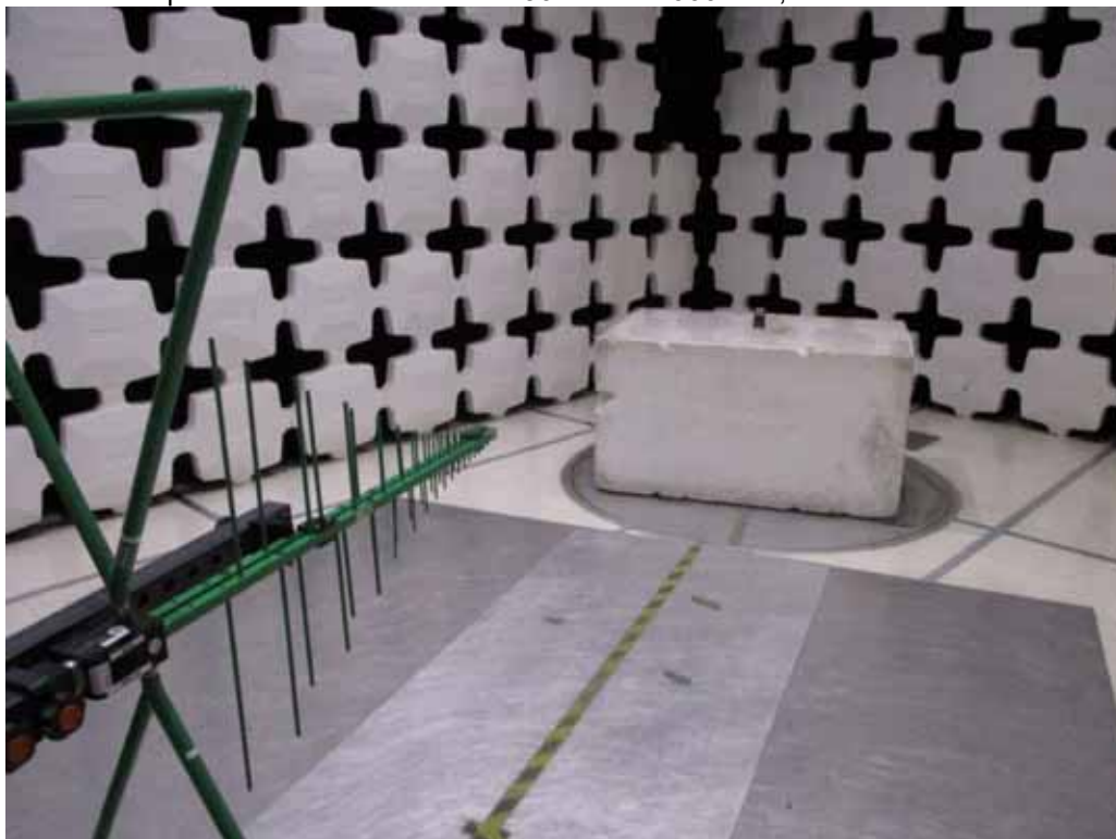
Test Setup for Radiated Emissions – 30MHz to 1000MHz, Vertical Polarization
