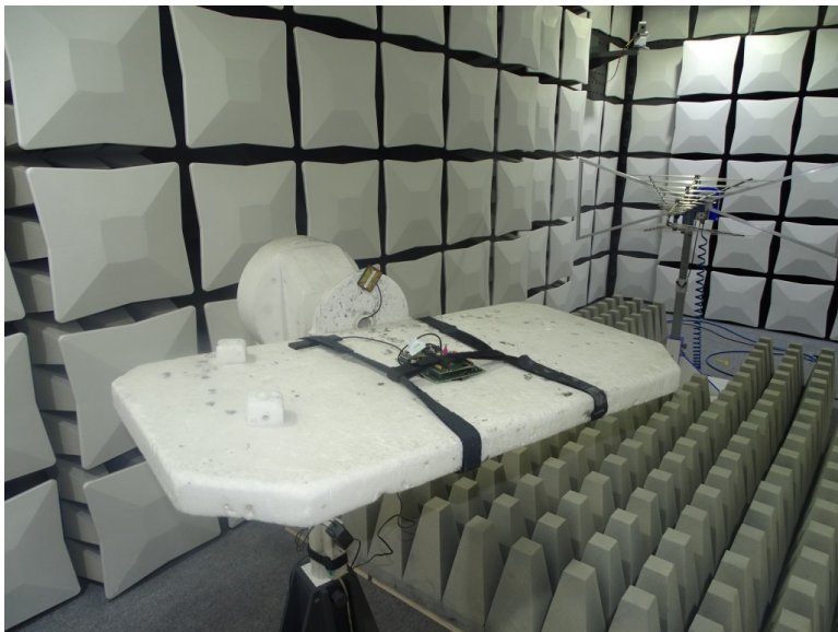
Photo 1: Test setup for radiated measurements below 1GHz
