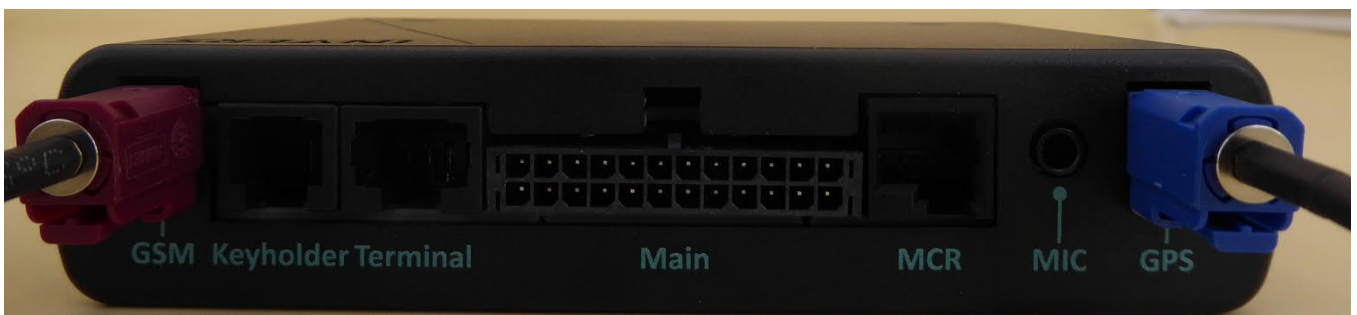
Rear Ports and antenna connectors
