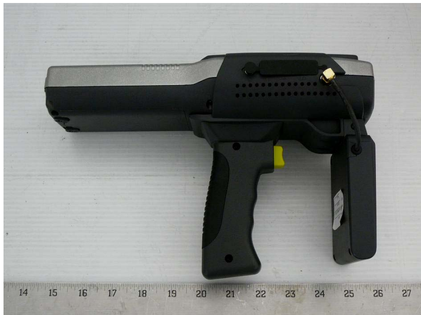
EUT with Holder and RFID Antenna
