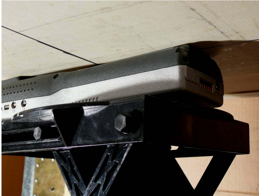
EUT Left Touch to Flat Phantom Setup Photo
