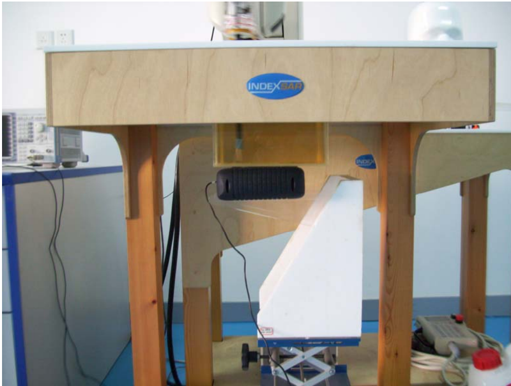
Fig.1 SARA2 System Test Layout
