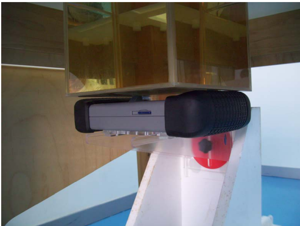
Fig.4 Test position_body Position (the EUT positioned against a flat phantom)
