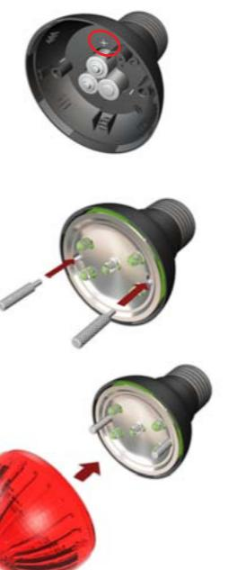
4. Please follow the image on the battery holder to install 3 x AAA battery (please note the orientation of battery).
