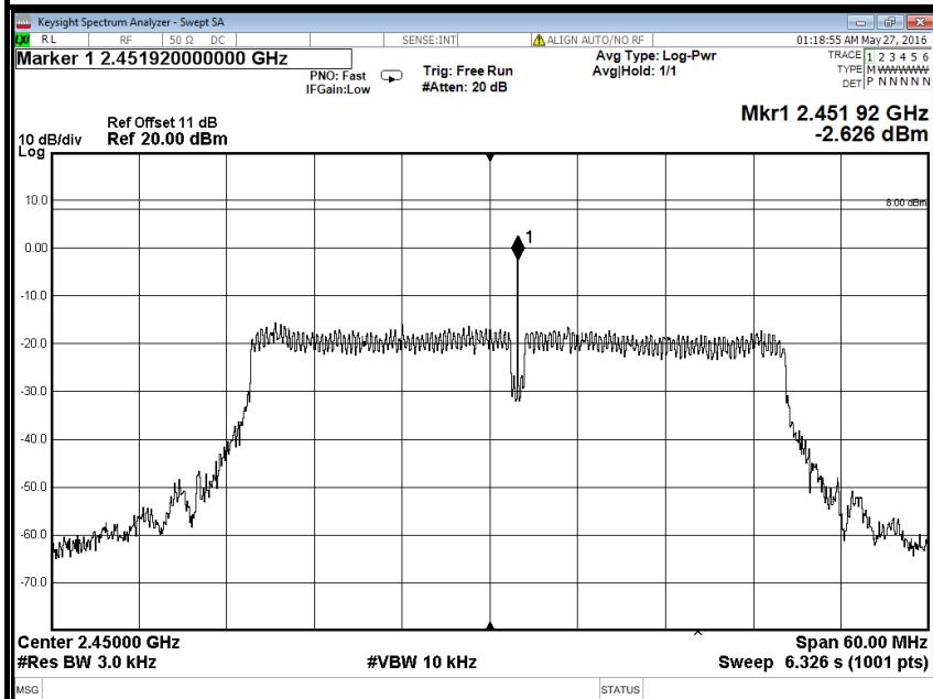
**IEEE 802.11n HT40 MHz mode (Antenna 2)****PPSD (CH Low)**
