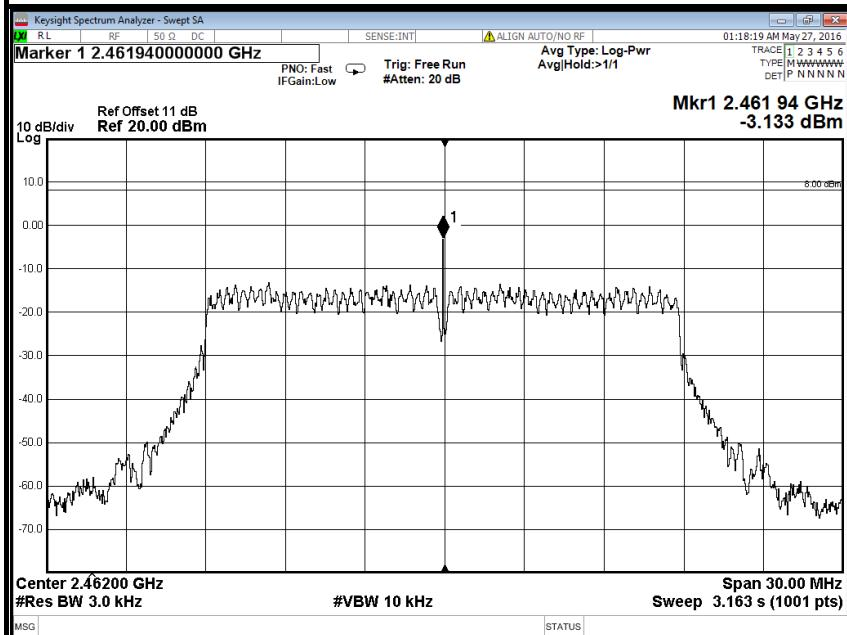
**IEEE 802.11n HT20 MHz mode (Antenna 2)****PPSD (CH Low)**
