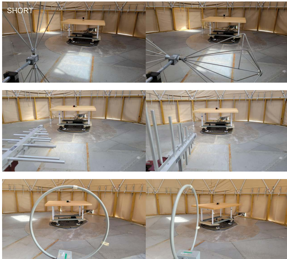
Figure 4.1.1 (i) Radiated Emissions Test Setup Photograph(s).
