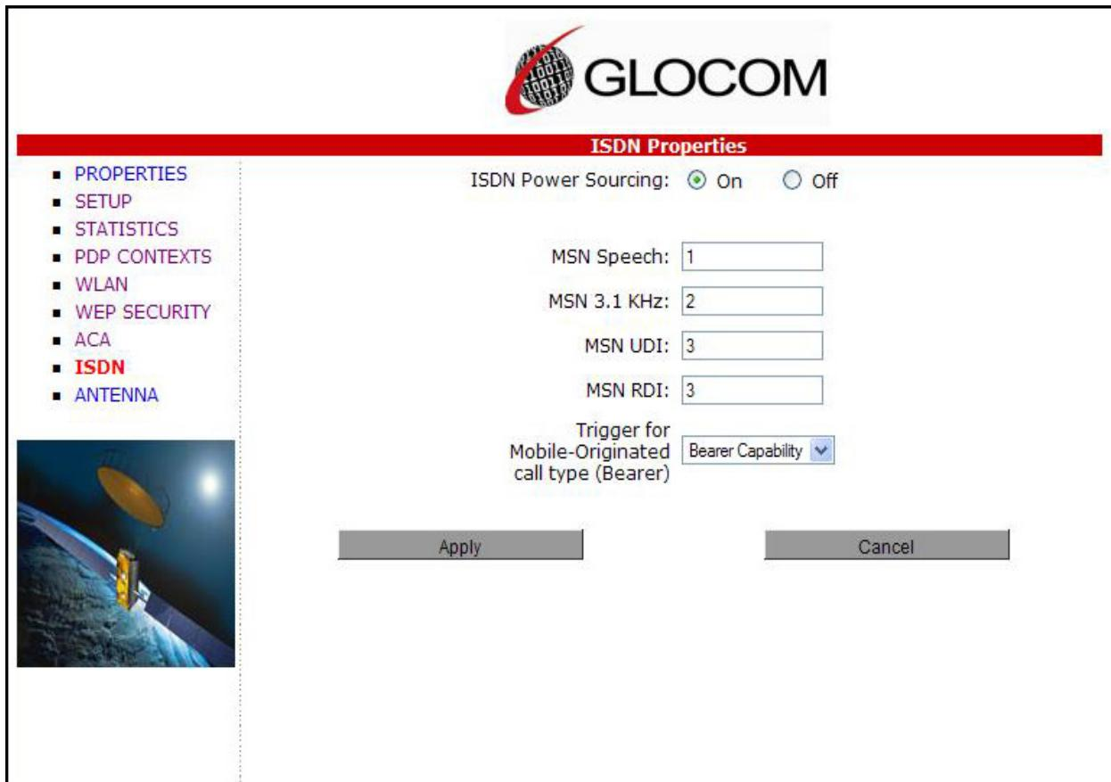
Once all changes have been made, click on “Apply”. Any changes to this screen require a re-boot of the terminal to save the new configuration. Use the power button on the UT or the “Restart Terminal” button to gracefully power down and power back up the UT.
