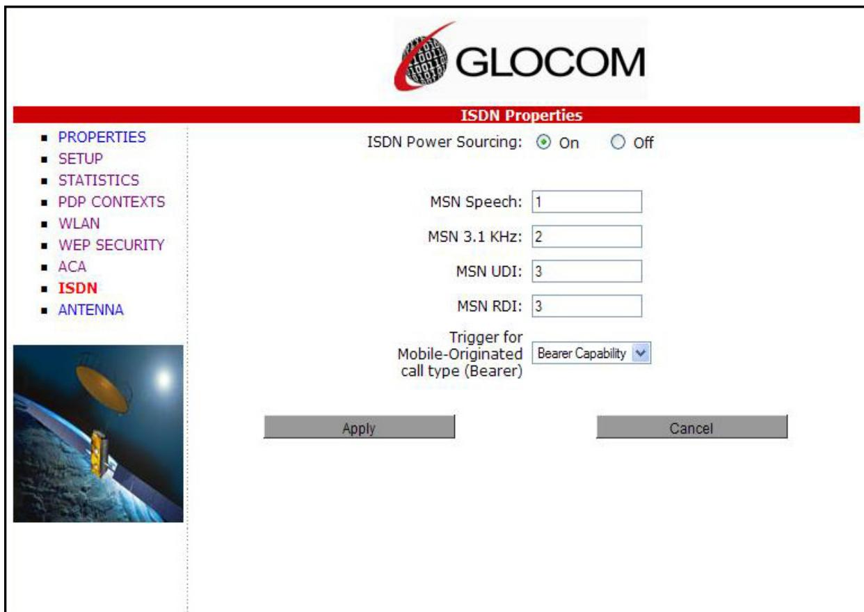
2. **ISDN Power Sourcing:** To turn on the ISDN power sourcing click on the “On” radio button. The ISDN device should receive 40V power immediately via the ISDN cable. This field should be on unless you never use ISDN or are using an ISDN device that has its own power source.
