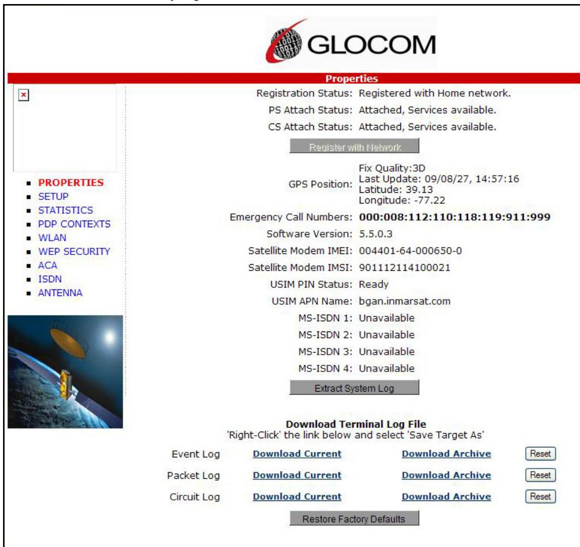
2. **PS Attach Status:** This indicates whether you are PS (Packet Switch) attached with the Network. You will still need to setup a PDP context in order to send PS data.
