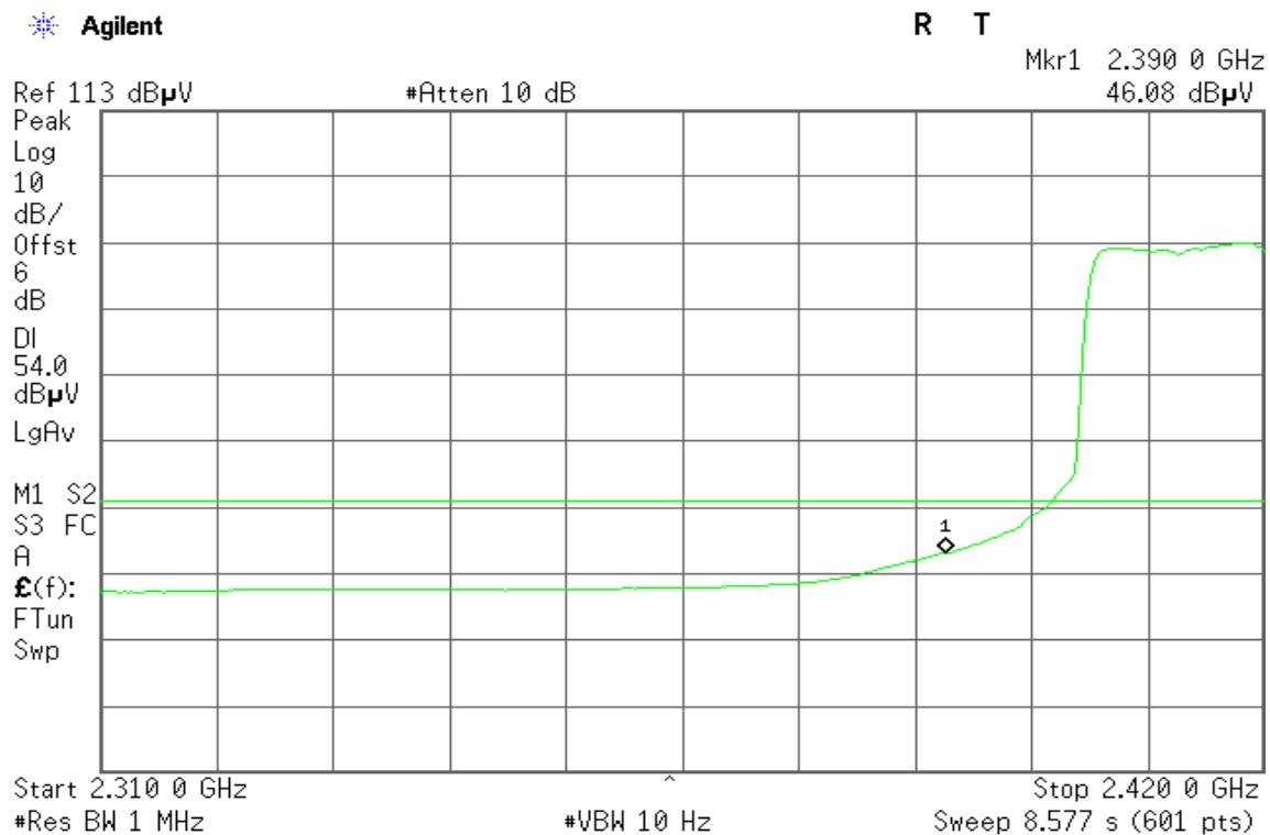
**Band Edges (IEEE 802.11g / CH High)****Detector mode: Peak****Polarity: Vertical**
