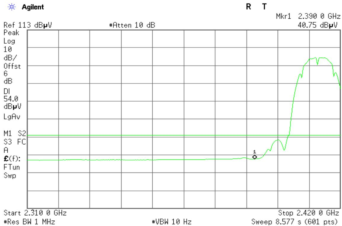
**Band Edges (IEEE 802.11b / CH High)****Detector mode: Peak****Polarity: Vertical**
