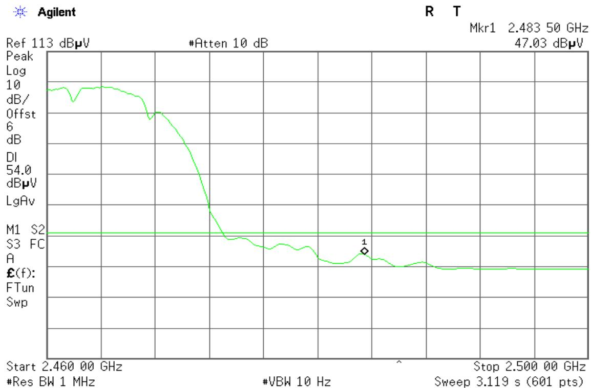
**Band Edges (IEEE 802.11g / CH Low)****Detector mode: Peak****Polarity: Vertical**
