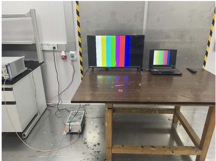
Conducted Emission Test Setup
