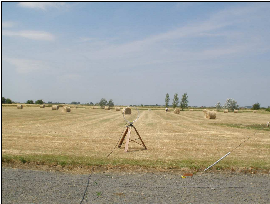
Photograph 3 Radiated Emissions - below 30MHz @ 100m
