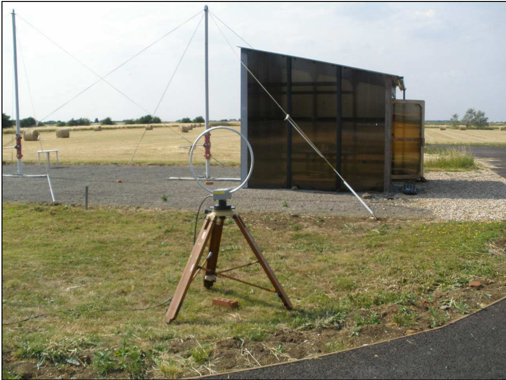
Photograph 1 Radiated Emissions - below 30MHz @10m
