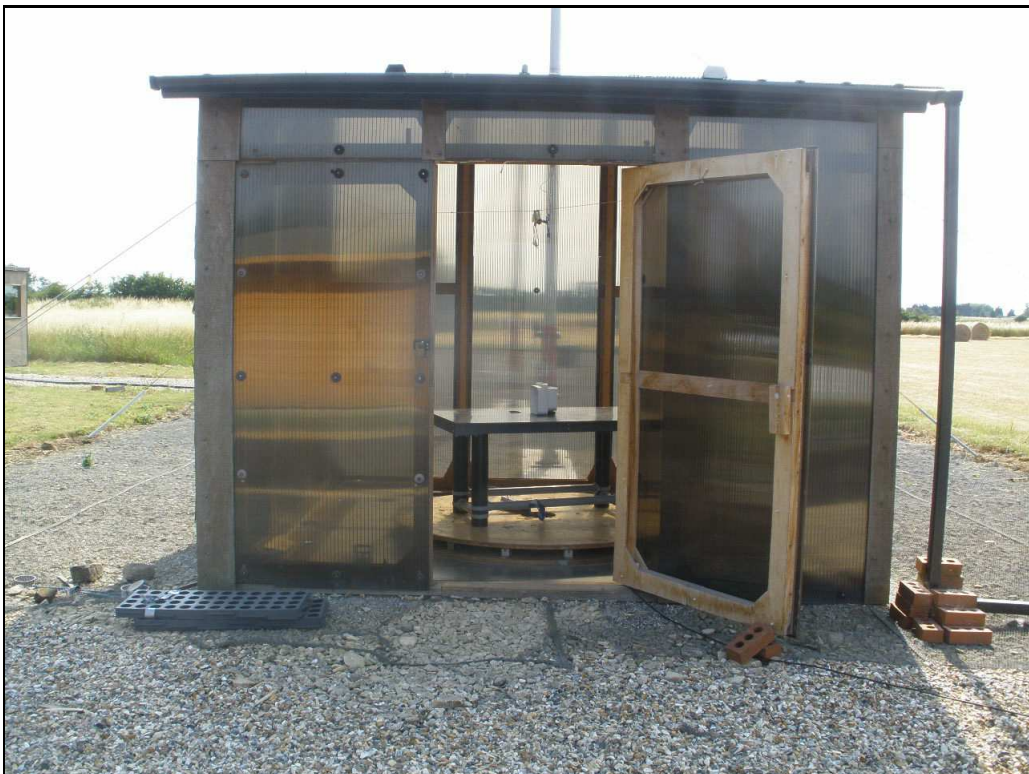
Photograph 2 Radiated Emissions - below 30MHz @10m
