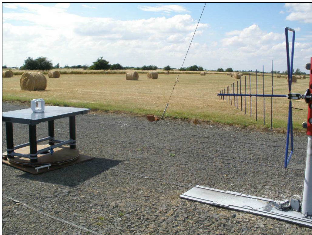
Photograph 4 Radiated Emissions - above 30MHz
