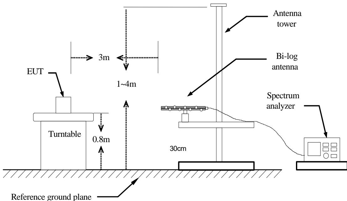
**Above 1 GHz**
