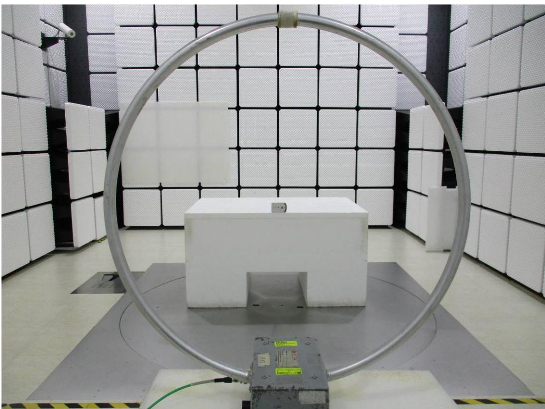
**RADIATED EMISSION MEASUREMENT SETUP(Below 1G)**
