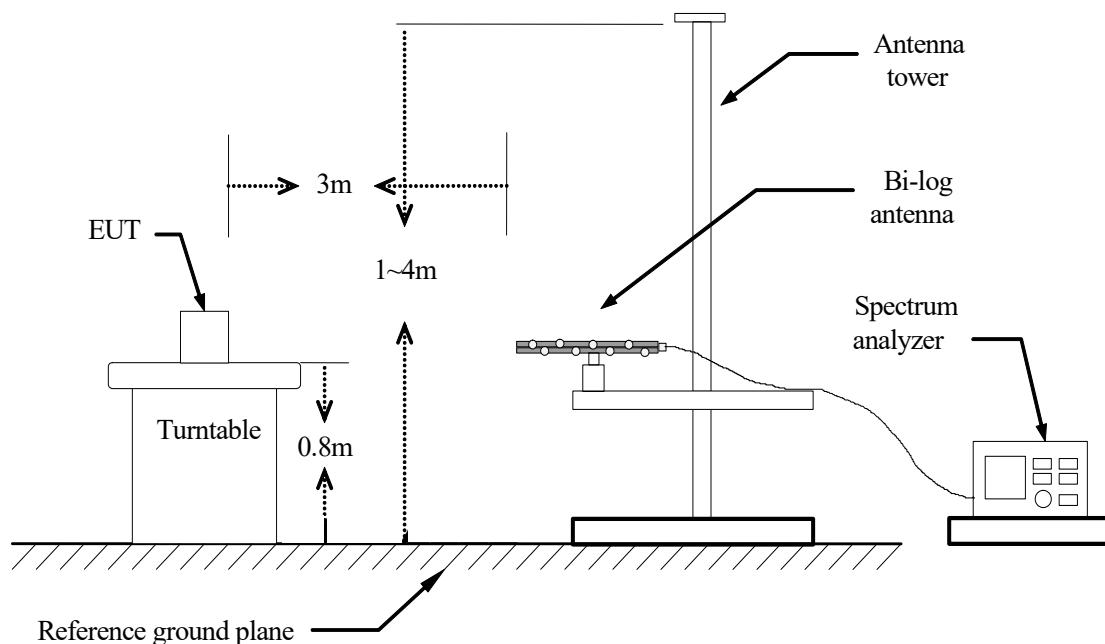
**Above 1 GHz**
