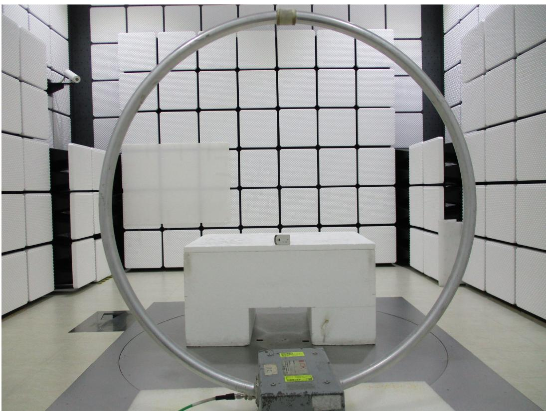
**RADIATED EMISSION MEASUREMENT SETUP(Below 1G)**
